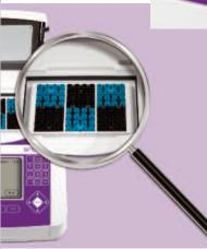
Intuitive user-friendly interface facilitates manual selection of different temperatures in each of the 4x4-well zones, for full user control during PCR optimisation.
